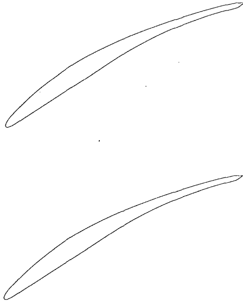
Fig. 17 Subsonic compressor cascade geometry (modified trailing edge)
